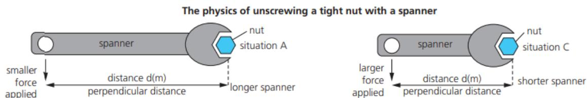
A **simple machine** makes it easier to lift things; they **reduce the force** needed
